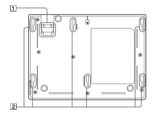
1Battery terminals (9)2Slots for the battery (9)
